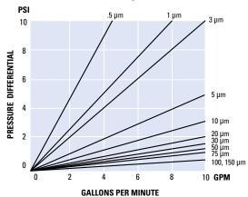
This chart represents the typical flow rate of polypropylene media per 10' cartridge length. The test fluid is water at ambient temperature. Extrapolations for multiple lengths tend to be linear, but as flows increase the differential pressure across the housing becomes more apparent.
